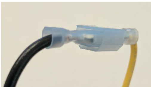
Figure 2 – Proper connection (male stab seated within female connector)
